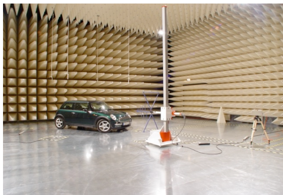
EMC facilities for radiated emission/susceptibility test
